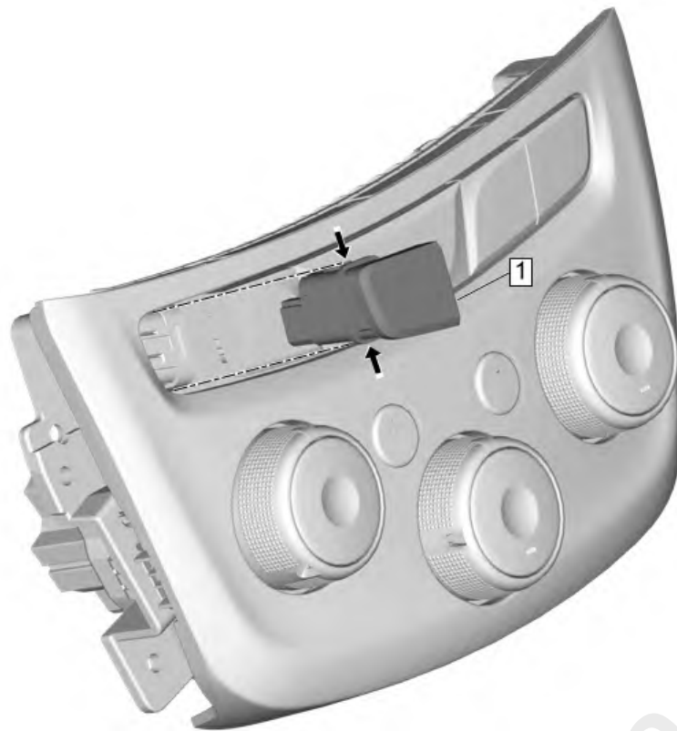
Fig. 45: Automatic Transmission Shift Program Switch (Blank Cover - Chevrolet). Courtesy of GENERAL MOTORS COMPANY
